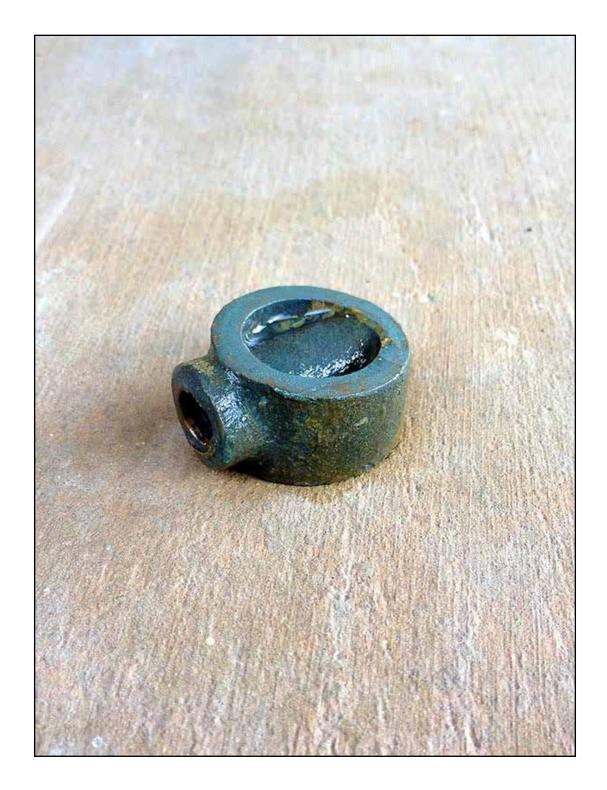
Above shows what the removed gate looks like. We were lucky to get this one out! Sometimes you're stuck and have no option but to immediately change out the valve. Gate Valves do have their place, but make sure you always replace residential home water valves with a high quality Ball Valve!
